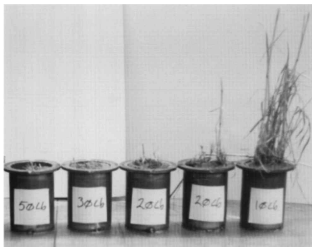
Fig. 3 Photographs of posttest VSU samples illustrating survival dependence on shock overpressure.
